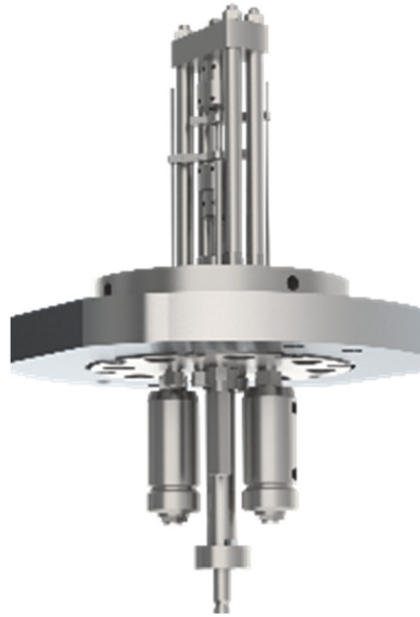
釜内直接测量试样应变 Direct testing strain in Autoclave
